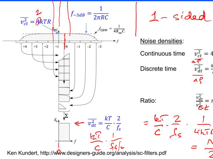
$\overline{v_{ct}^2} = 4kTR$  $\frac{\overline{k}}{v_{dt}^2} = \frac{kT}{c} \cdot \frac{2}{f_s}$  $\frac{\overline{v_{dt}^2}}{\overline{v_{dt}^2}} = \pi \frac{f_{-3dB}}{f_s} \gg 1$ C fs 4hrR 2fs Rc
