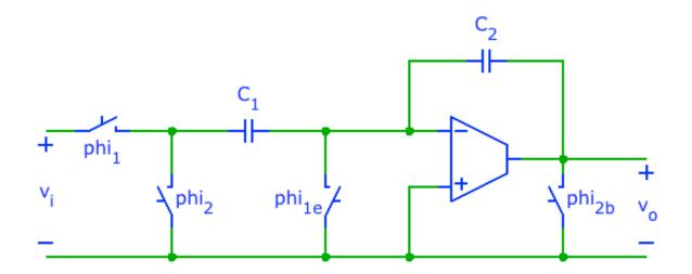
Switches controlled from non-overlapping 2-phase clock:
